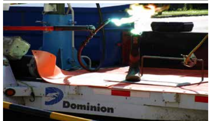
Demonstration of how rubber boots do not provide insulation from arcing electricity.
